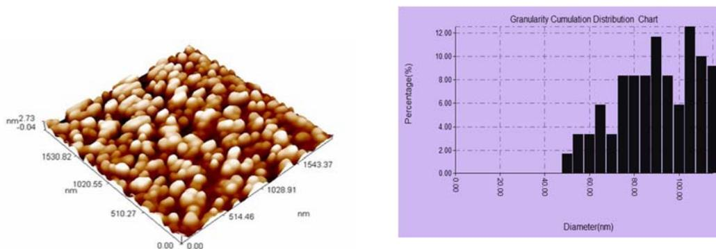
Figure (4): AFM images and diameter allocation of Nano crystalline cellulose.
