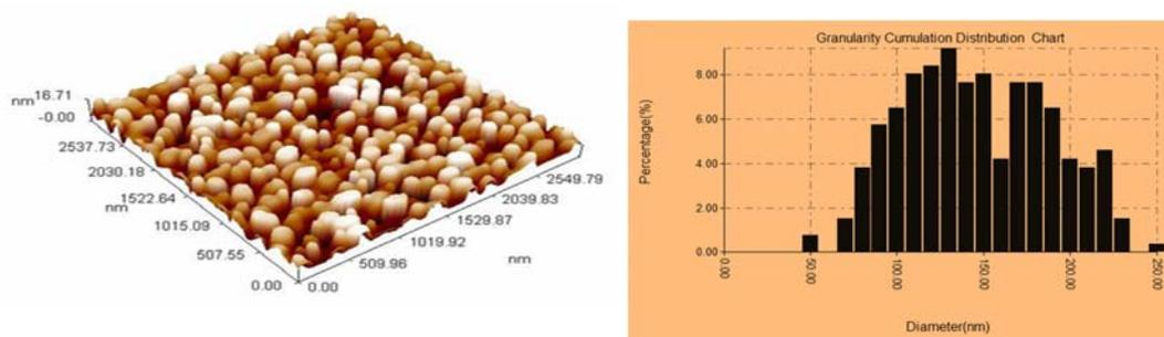
Figure (3) : AFM images and diameter allocation of microcrystalline cellulose
