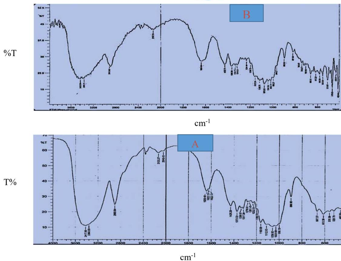
Figure (2): (B) FT-IR spectra of microcrystalline cellulose, (A) FTIR spectra of Nano crystalline cellulose
