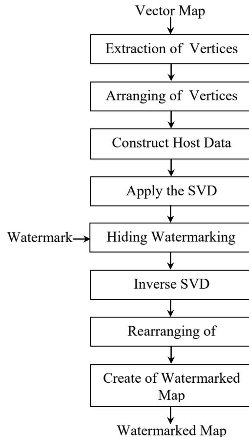
**Figure (1): The hiding model of proposed scheme.**
