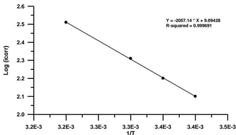
Figure (2): Plotting  $\text{Log}(i_{\text{corr}})$  vs  $1/T$  for the corrosion of pure Al in the  $\text{pH} = 0.7$  in presence of  $(0.6 \text{ mol.dm}^{-3})$  NaCl over the temperature range (293 – 308) K.
